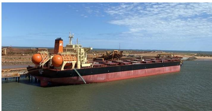
*Bulk carrier cu system propulsive dual fuel LNG- MGO.*
