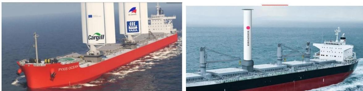
Mitsubishi Corporation's Pyxis Ocean is set to be the first vessel fitted with BAR Technologies' wind propulsion technology WindWings.
